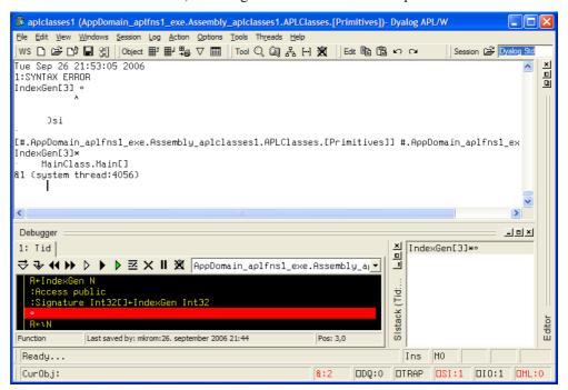
Notice too that IndexGen has been started on APL thread 1 which, in this case, is associated with system thread 4056. If the client application were to call IndexGen on multiple system threads, this would be reflected by multiple APL threads in the workspace. This topic is discussed in further detail below.
